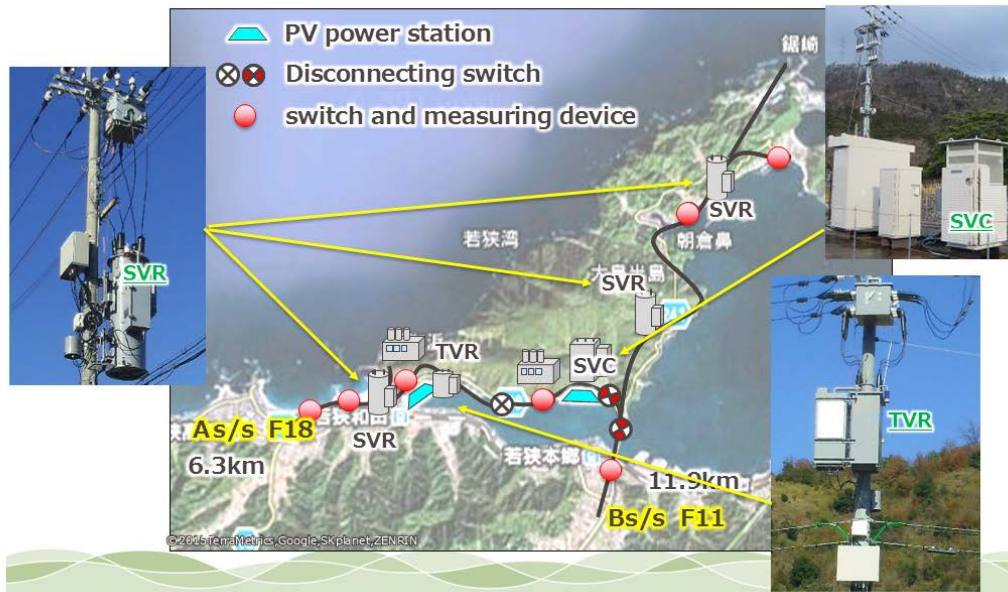
Fig. 2-50 System components (SVR)
